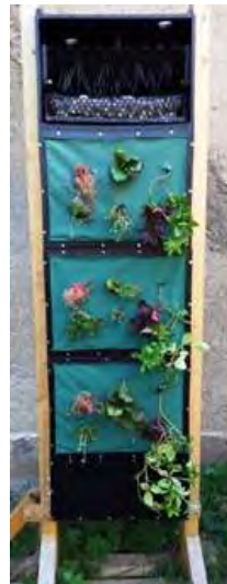
Test installation with expanded granulate (right) and rock wool (left)
